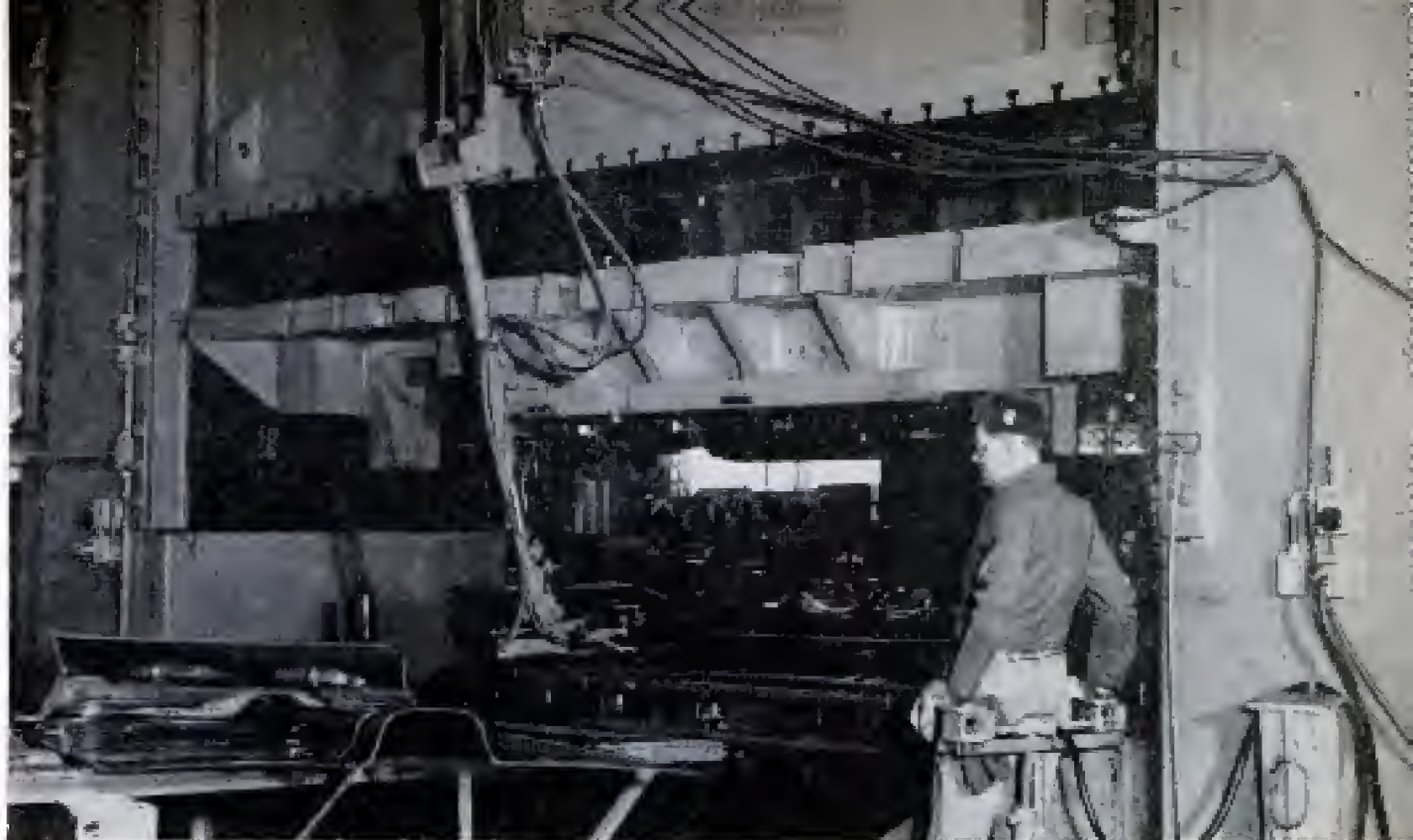
Pneumatic "iron hand" reaches into a big press, snatches a sheet of steel and deposits it on a conveyor
